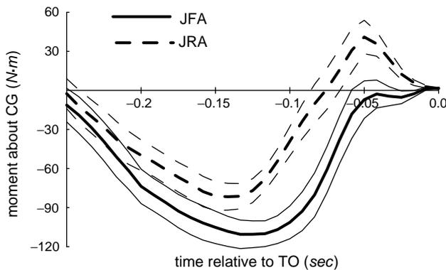
Fig. 5. Moment profiles of the GRF about the CG for the last 0.25 s before TO for both JFA and JRA (LSM  $\pm$  95% CI). Subjects generated greater positive (pitching backward) and negative (pitching forward) magnitudes of the moment about the CG for JFA. A counterproductive backward-pitching moment is generated over the last 0.075 s before TO for JRA.
